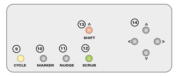
The marker control (10) can be used to add memory locations to the marker track in Pro Tools. This may be useful for flagging edit points during a take for example. Tap on the marker switch to place a marker in the timeline, a second tap will close the
