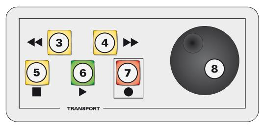
When operating the rewind or fast-forward controls (3 & 4) it should be noted that one switch press (released immediately) initiates a playhead movement of one bar or second etc depending upon which ruler is currently active in Pro Tools.
