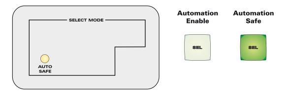
Note that all select mode layers are stored and function simultaneously. By toggling the select mode switches in conjunction with the large green channel select switches it is possible to obtain rapid control of SIP safe, DAW record enable, select, unity and automation safe channel settings.
