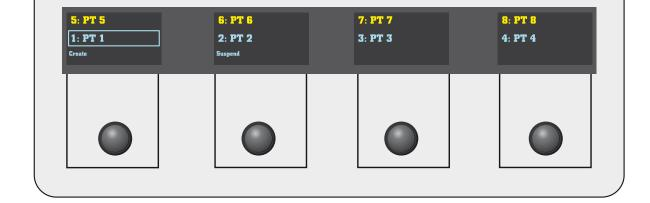
Select the tracks you wish to group by holding down and pressing multiple channel select switches (18) at once.
