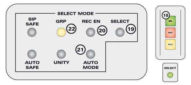
When select mode is chosen (19), the large green channel select switches above the channel faders become DAW channel selects when in control surface mode. Selected channels are highlighted in white within Pro Tools and a box is shown around the channel name in the ASP2802 OLED display. Multiple channels can be added or removed from larger selections by holding down one or more select switches at once and pressing other channels to add or remove.
