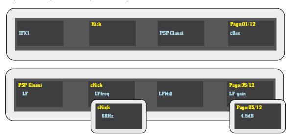
The OLEDs will display parameter values during encoder rotation but after a few seconds will return to displaying the parameter title.
