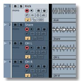
Please note that by using multiple channel select switches (18), you can record enable more than one track at once.
