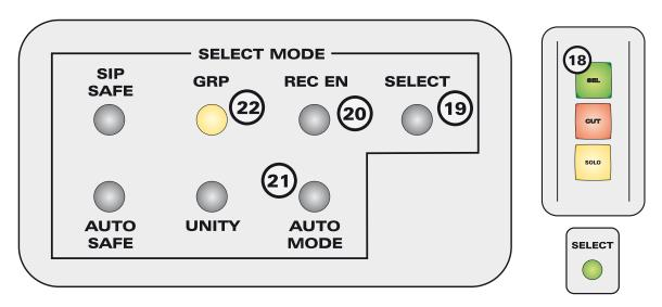
When select mode is chosen (19), the large green channel select switches above the channel faders become DAW channel selects when in control surface mode. Selected channels are highlighted in light grey within Cubase / Nuendo and a box is shown around the channel name in the ASP2802 OLED display. In Cubase / Nuendo, only one channel can be selected at any one time from the hardware but shift+clicking in software allows multiple selections.
