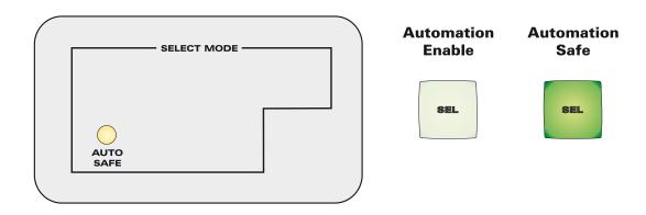
Note that all select mode layers are stored and function simultaneously. By toggling the select mode switches in conjunction with the large green channel select switches it is possible to obtain rapid control of SIP safe, DAW record enable, select, unity and automation safe channel settings.
