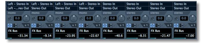
Rotate the encoders to change level, press on them to toggle between send on / off and pre / post fader settings.
