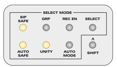
Automation Safe - used in the analogue layer for isolating channels from any automation control data, ideal for trying out a new ride before recording the pass of automation.
