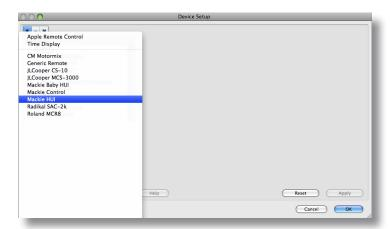
**Step 4**: Here assign the MIDI inputs and outputs to the ASP2802 Control Surface ports in the drop down menu.
