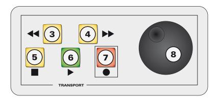
When operating the rewind or fast-forward controls (3 & 4) it should be noted that one switch press initiates a small jump in either direction and you must press and hold either switch to perform playhead rewind or fast-forward. Releasing the switches will return to the previous mode of operation (stop or play).
