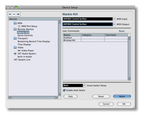
You should be ready to go, please enter DAW layer on the ASP2802 and ensure that it picks up your channels in Cubase / Nuendo and you can bank around the project using the channel bank or nudge keys in the controls surface,
