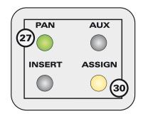
Input assigns are set on page one. Use the page keys (26) to access page two where polarity reverse can be toggled on and off.
